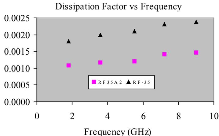
All reported values are typical and should not be used for specification purposes. In all instances, the user shall determine suitability in any given application. Test data obtained using a 0.0600" sample and 5 and 10 mil building blocks where indicated.
